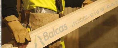
Tanalith® E pressure treated timber is timber which has been impregnated with Tanalith® E wood preservative under controlled conditions in a vacuum pressure timber impregnation plant.
